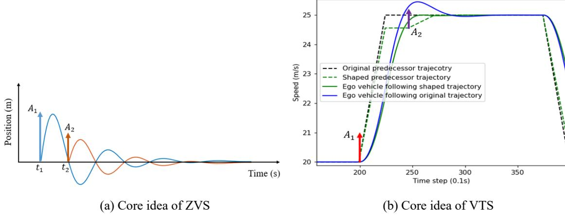
Figure 2 - Core ideas of ZVS and VTS
