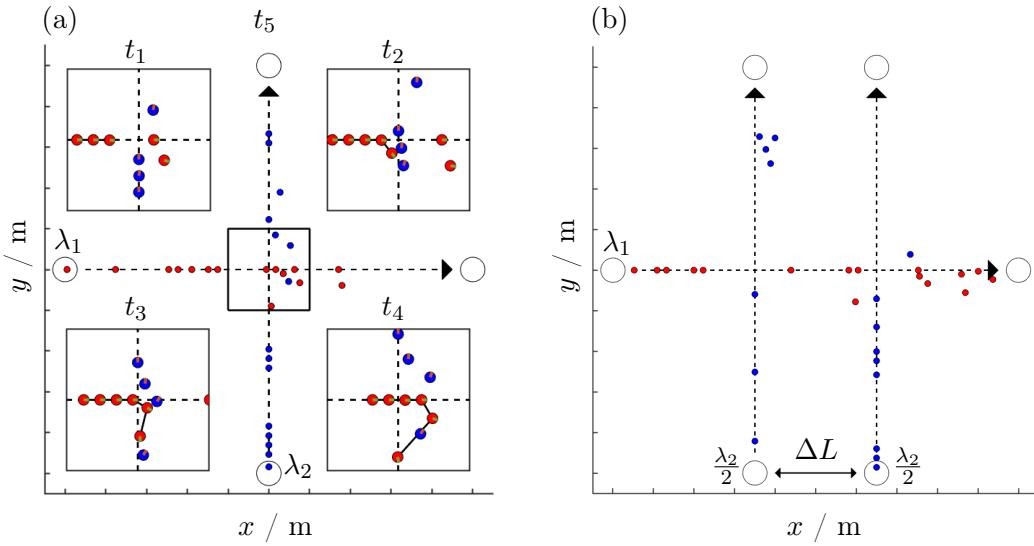
Figure 1 – (a) Two streams of autonomous UAV traffic, described by take off rates  $\lambda_1$  and  $\lambda_2$  from the origin ports, form a crossroads and use a S&A method to resolve future conflicts. (b) The vertical traffic stream (as viewed on the page) in (a) has been split in to two parallel streams,  $\Delta L$  apart, that equally share the demand of the single stream. Thus the number of crossings has increased but the contention at each is reduced.
