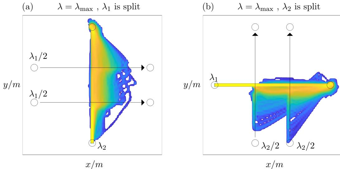
Figure 3 – Time aggregated density plots for traffic in the (a) vertical stream when the horizontal stream is split and (b) horizontal stream when the vertical stream is split. In both scenarios the traffic in the un-split stream is dispersed laterally so that the contention at the second crossroads it encounters is reduced.
